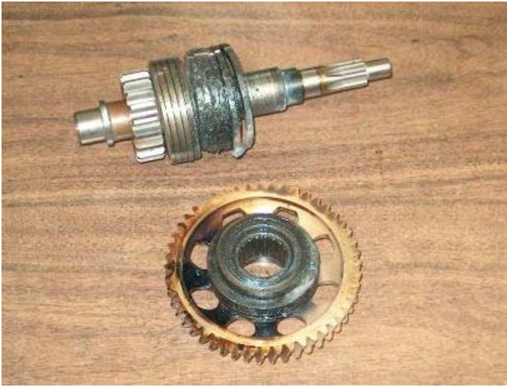
STARTER NOT OVERHAULED / CLUTCH SPRING FAILED TO RELEASE
